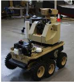
Figure 4: LandShark unmanned ground vehicle; (a) The vehicle; (b) Coordinate system and variables used to derive the model; (c) Control system diagram used for cruise control.
