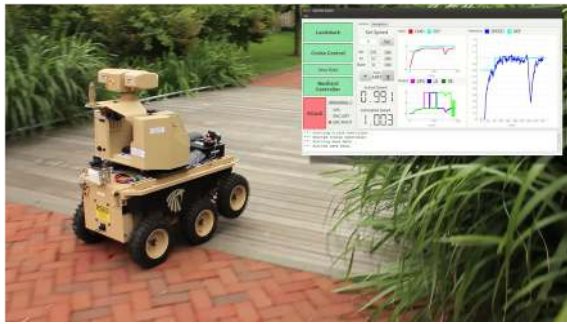
Figure 5: Deployment of the LandShark on a tiled pathway. The picture in the picture displays the user interface used in experiments.
