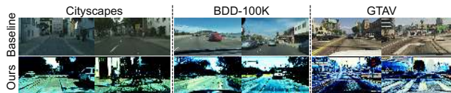
Figure 7. Reconstructed images from ISW-whitened feature maps using U-Net; the first row: a baseline backbone, the second row: an ISW model backbone. The image contents are properly maintained while the style such as illumination and colors vanish.
