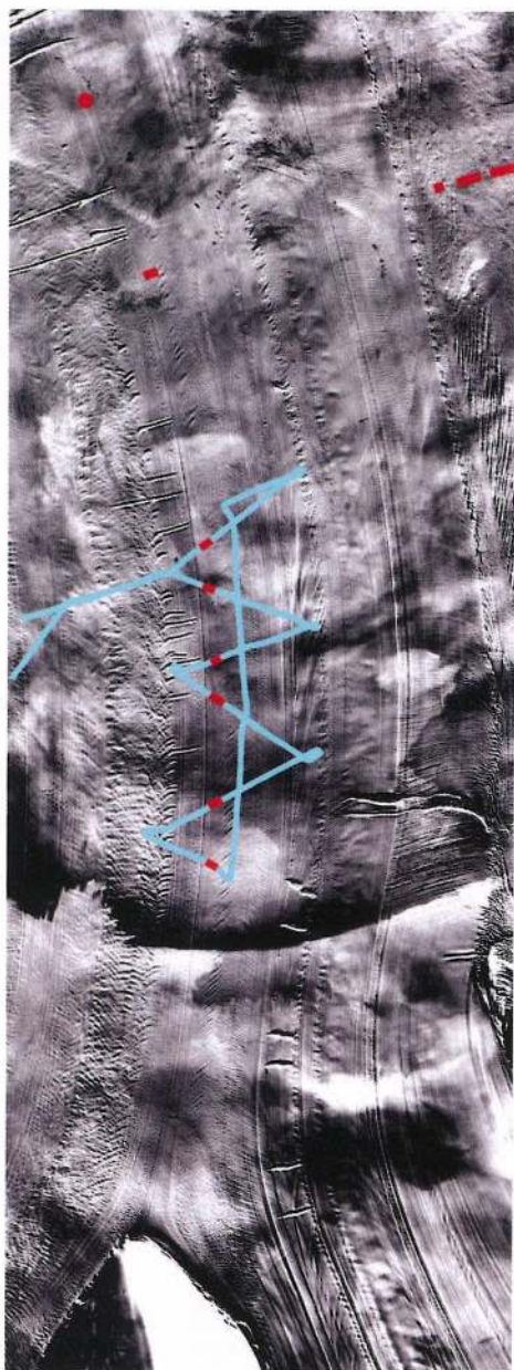
Fig. 5. Satellite image rendered to highlight the surface features, and indicate the route and likely source of the debris found at Fox 4 (red dot at top of picture). The radar flight-line is shown in cyan, with the red portions indicating the location of bright reflectors. Bright reflectors in one of the 1982/83 flight-lines are also shown. Fowler Peninsula is visible at the bottom of the picture.
