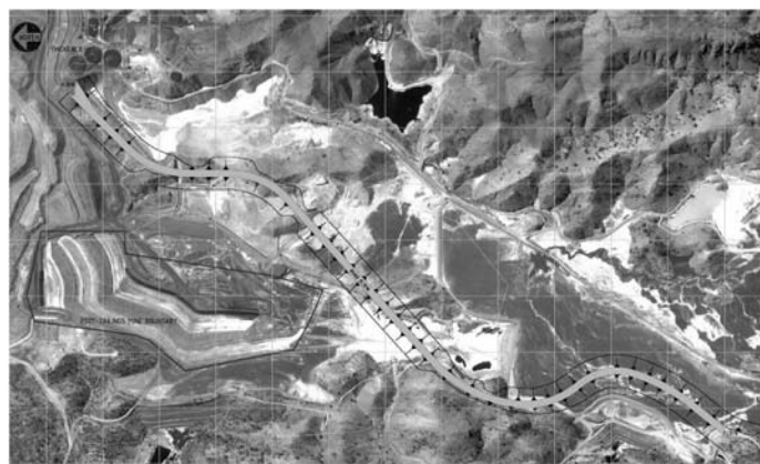
Figure 2 Proposed outfall groyne tailings TSF No. 5
