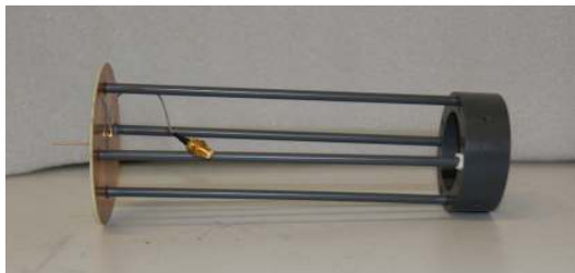
Fig.5. Monopole antenna mounted on the support pole.
