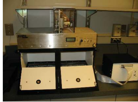
FIGURE 2: Passive avoidance: the mice are trained to avoid the preferred dark compartment by pairing it with an aversive stimulus.
