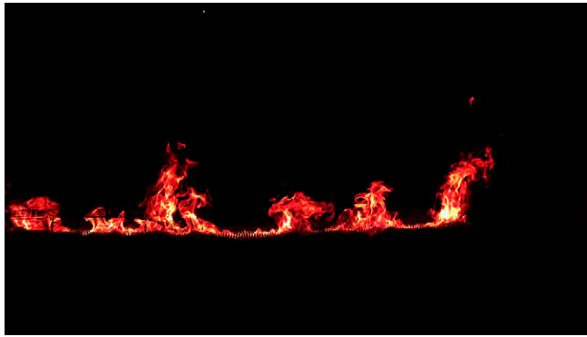
Movie S5. Wide-angle view from high-speed movie shows peak and trough structure of 0.2-m flames at the leading edge of an approaching fire in the MFSL wind tunnel burning engineered cardboard fuel bed.
