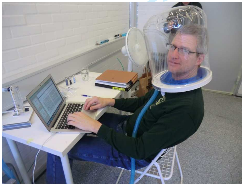
Figure S1. Male subject shown wearing full set of test clothing and the breathing hood while seated in the test chamber.
