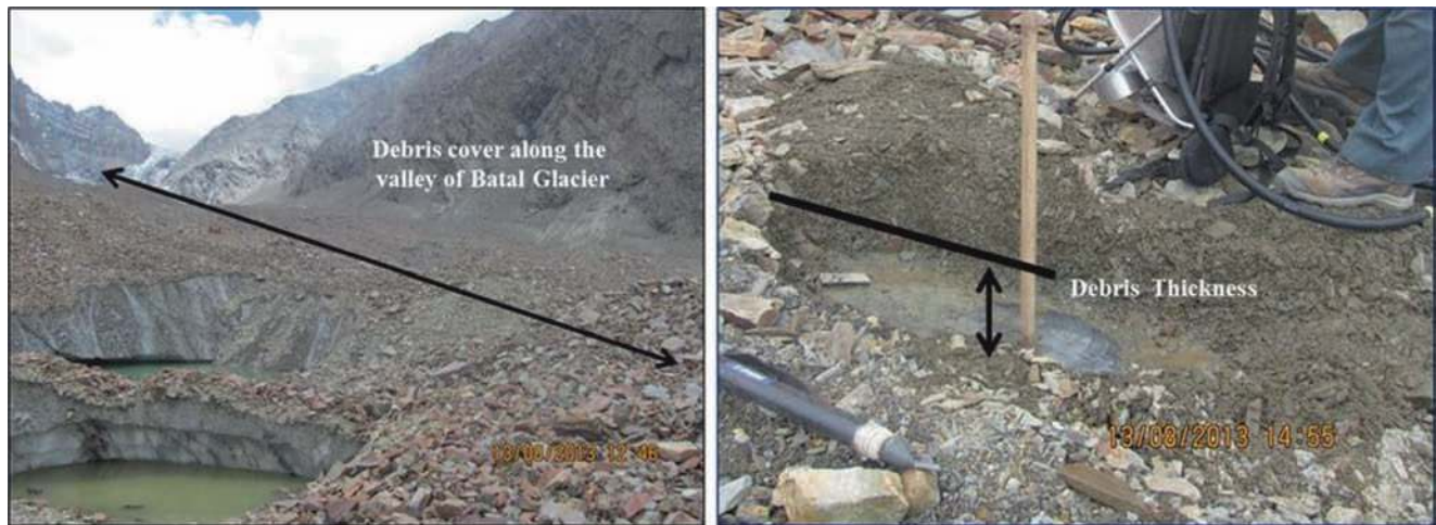
Figure 5. Field photographs showing in situ observation of debris cover and manual measurements of debris thickness.
