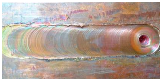
Figure 4. Typical crown appearance of friction stir processed copper using B 4 C particles.
