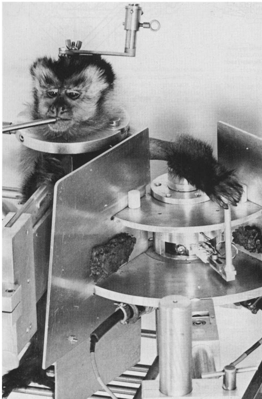
Figure 5—A Cebus monkey in the task situation. The animal is restrained in the chair by a neck collar and head holder. A juice reward delivery tube is in front of the mouth. The left elbow rests on a rotatable pivot, and the hand grasps the knob of the handle, which is connected to a potentiometer and torque motor. Not shown are opaque plate that blocks monkey's view of his arm, and the microdrive for recording in motor cortex.
