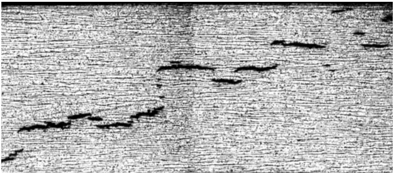
Figure 12 - HIC in an ASTM A516-70 plate steel. Note crack parallel to plate surface and ferrite/pearlite bands.
