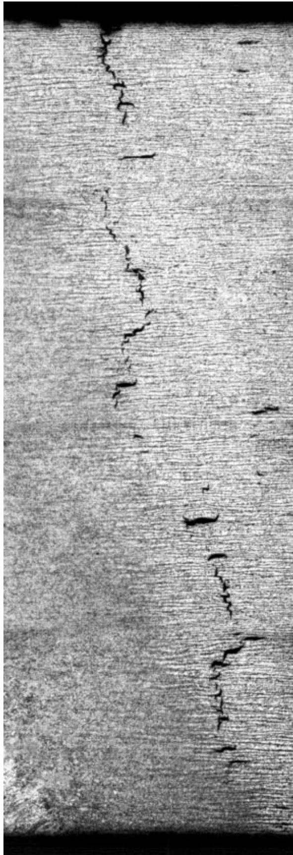
Figure 13 - SOHIC in the base metal adjacent to a weld heat affected zone on an ASTM A516-70 plate steel.
