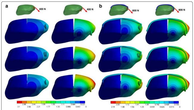
Fig. 2 Total deformation (mm) of the fractured patella under a loading force in a direction 45° to the long axis of patella without (a) and with (b) the wire. The top, middle and bottom row is the full thread, headless compression and partial thread screw, respectively
