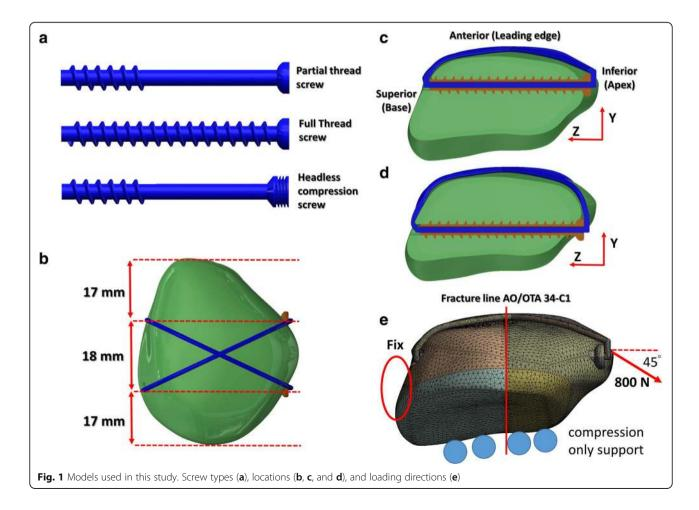
modulus and Poisson ratio were set to 210 GPa and 0.3, respectively; In the plastic stage, the yield strength and tangent modulus were set to 250 MPa and 1450 MPa, respectively.
