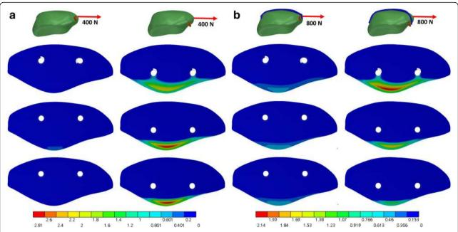
Fig. 5 Contact pressure (MPa) of the fracture site under a loading force in a direction parallel to the long axis of the patella without (a) and with (b) the wire. The top, middle and bottom row is the full thread, headless compression and partial thread screw, respectively
