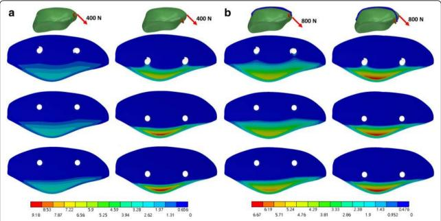
Fig. 4 Contact pressure (MPa) of the fracture site under a loading force in a direction 45° to the long axis of the patella without (a) and with (b) the wire. The top, middle and bottom row is the full thread, headless compression and partial thread screw, respectively
