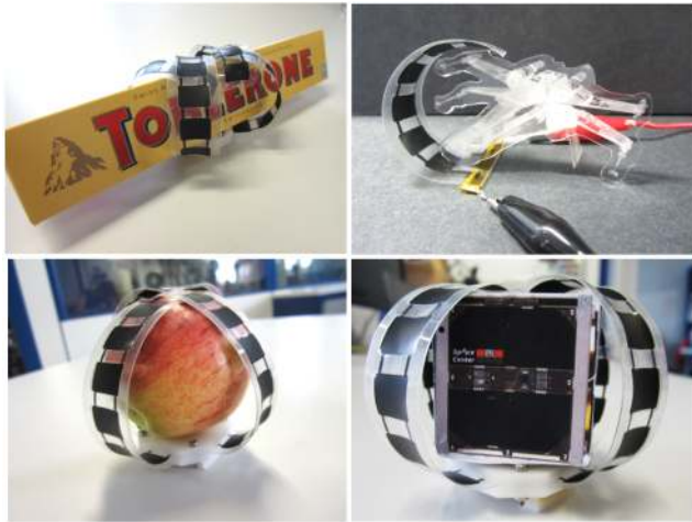
Fig. 8. Fabricated DEMES actuators wrapped around objects of various shapes and sizes to demonstrate conformability. Objects are (from left to right, top to bottom): Toblerone bar, PMMA piece laser cut into the shape of a fictional spacecraft, an apple, a model of SwissCube.
