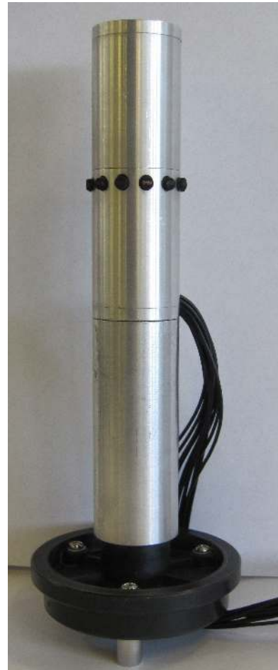
Figure 3: This figure shows a photo of the 12 sensor cylindrical microphone array used for the room measurements.
