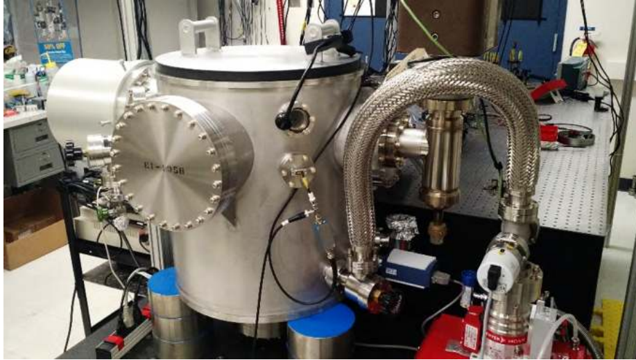
Figure 5-3: Vacuum chamber that contains the main Fabry-Perot cavity of the experiment. The vacuum chamber is placed on top of three stacks of steel masses sandwiched with high damping material (blue disks). This view shows the side-imaging port on the left of the chamber. The 2.75 inch flange supporting the window for external illumination for the side imaging can be seen above the flange connected to the turbo pump.
