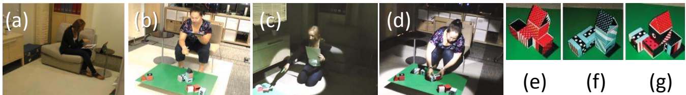
Figure 6: Experimental task setup: (a) Instructor in Skype condition. (b) Assembler in Skype condition assembling a shape based on her partner’s instructions. (c) Instructor in Room2Room condition; note the virtual copy of the task space projected in front of her. (d) Assembler performing the task in Room2Room condition. (e-g) Target shapes used in the assembly task.
