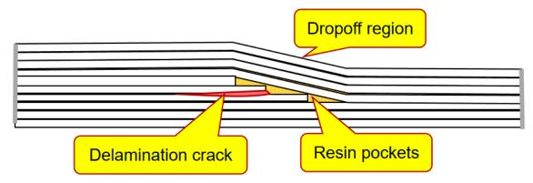
Figure 5. Schema of a delamination crack in the plydrop region.
