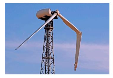
**Figure 1.** Wind turbine with broken blades. The photo from Bigstock<sup>©</sup> collection is reproduced according to the Bigstock content usage agreement.
