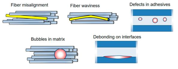
**Figure 8.** Schema of the typical manufacturing defects on wind turbine blade composites: fiber misalignment and waviness, voids in adhesives and in matrix, debonding on interfaces.
