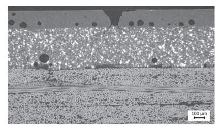
**Figure 9.** Voids in leading edge protection layers: Sites of damage initiation. Reprinted from [15] with kind permission from Wiley.
