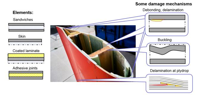
**Figure 7.** Elements of the blade structure (**left**), blade cross section (**middle**) and some common damage mechanisms (**right**). On the blade cross section, white adhesive layers and brown/white sandwiches can be seen. The photo from Bigstock<sup>©</sup> collection is reproduced according to Bigstock standard content usage agreement.
