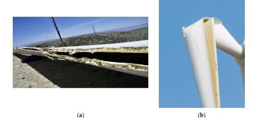
**Figure 6.** Blade failure: (**a**) Failure of edges in 24 m wind turbine blade. Reprinted from [27,84] with kind permission from Elsevier, and (**b**) Collapsed blade.
