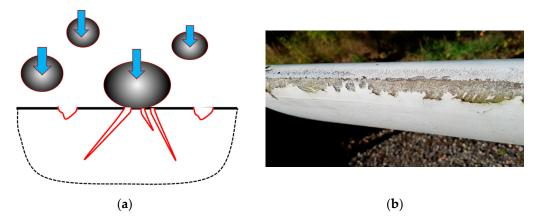
Figure 4. Schema of leading edge erosion of blades (a) and eroded blade (b).
