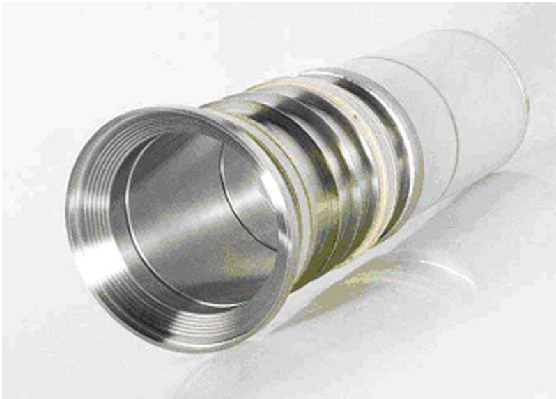
Figure 17. The integrated reflectron consists of an electrostatic lens in the entrance area and two following resistive helix segments, which generate the retarding and repelling potentials. The ions loose about two-thirds of their energy in the short retarding region and turn around close to the solid backplane. (a) Schematic of the reflectron and (b) the EQM integrated reflectron.
