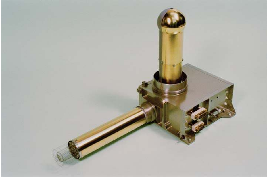
Figure 23. Picture of the ROSINA COPS-FS. The nude gauge is pointing to the left and the ram gauge is mounted on the top of the electronics housing. Connectors (with connector-savers) to the DPU are fitted into the right panel of the electronics box.
