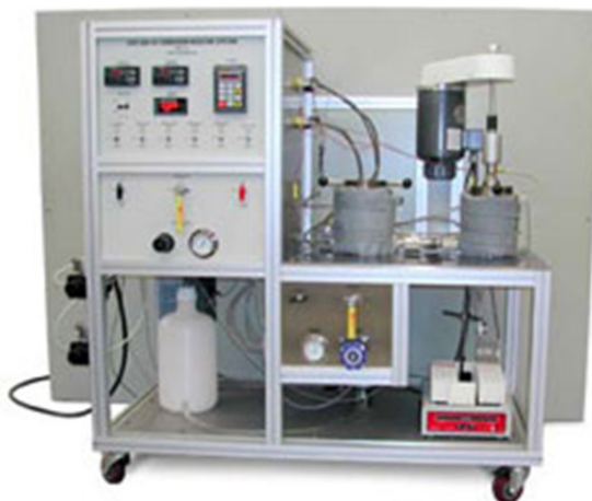
Figure 4. The rotating disk acid reaction system (CRS-100)
