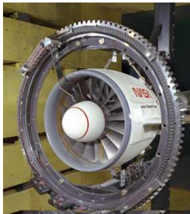
Figure 11.—Rotating rake ring assembly on geared advanced ducted propulsor in the 9- by 15-foot wind tunnel.
