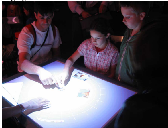
Figure 1. A multi-user, direct-touch table system. Each participant has a unique perspective, necessitating dynamic reorientation of objects.
