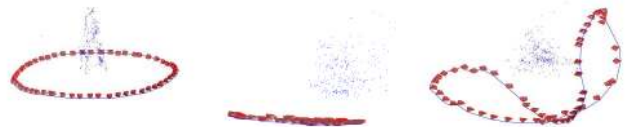
Figure 1: In many structure from motion pipelines, camera orientations are estimated with rotation averaging followed by recovery of camera centres (red) and 3D structure (blue). Here are three solutions corresponding to different local minima of the same rotation averaging problem.
