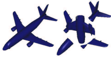
Figure 5: The model on the right is obtained by applying a rotation to the interior part of the model on the left. While the models differ by more than a single rotation, their rotation invariant representations are the same.
