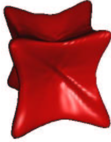
Figure 9: The Radial Variance can be visualized by displacing the radius at a point on the sphere, in proportion to the value of the function at that point.
