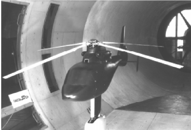
Figure 1: Dauphine Model in S2Ch Wind Tunnel
