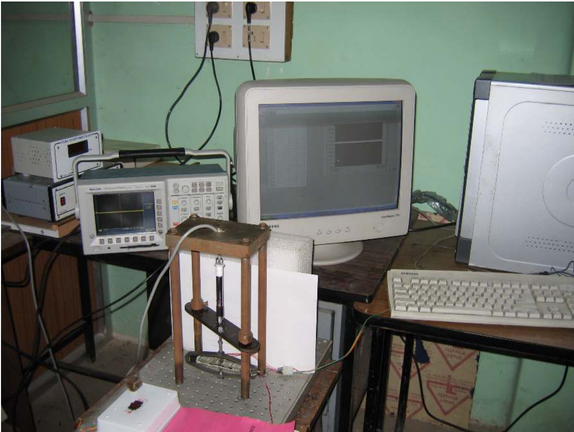
Figure 9 Picture of experimental facility used for evaluating the dynamic hysteresis behavior of the piezostack actuator
