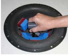
Fig. 2. Subject's hand on the manipulandum of the magnetic levitation haptic device.
