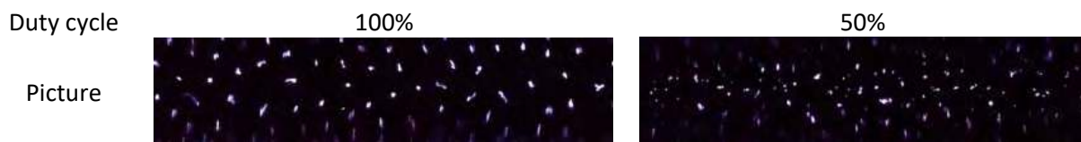
Figure 14: Pictures of the distribution of the microdischarges in the DBD for 100 and 50% duty cycle. P_{applied} = 50 \text{ W} , f_{signal} = 28.6 \text{ kHz} and \Phi(\text{CO}_2) = 200 \text{ mL}_n \cdot \text{min}^{-1} . Camera aperture is 1/100 \text{ s} .
