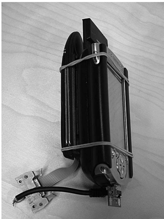
Figure 8. The sensor box attached to a PDA.
