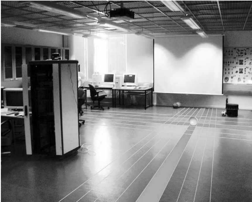
Figure 10. The setting for EMFi sensor strips under the laboratory's normal flooring.
