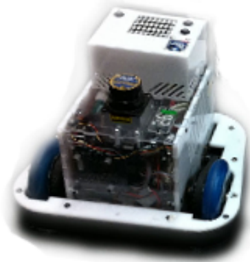
Fig. 5. Scarab robot used in experiments. It is capable of self-localization and point-to-point radio signal strength measurements with an off-the-shelf Zigbee radio.
