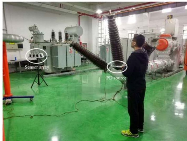
Figure 8. Sensor array in the high voltage (HV) laboratory.
