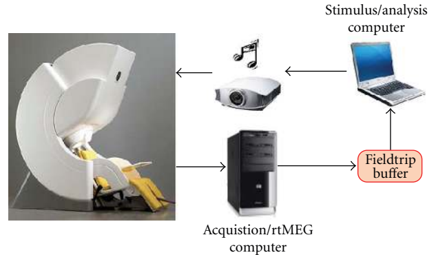
FIGURE 1: Illustration of a typical setup with rtMEG. The acquisition computer controls the acquisition, stores the data, and runs the rtMEG interface. Another computer drives the experimental paradigm by providing stimuli to the subject and sending trigger events that eventually go to the MEG data file. The rtMEG interface writes data to the Fieldtrip buffer, which can be run by rtMEG or by any other computer in the network. The application(s) reading from this buffer can run on the stimulus computer or on any other computer connected in the network.
