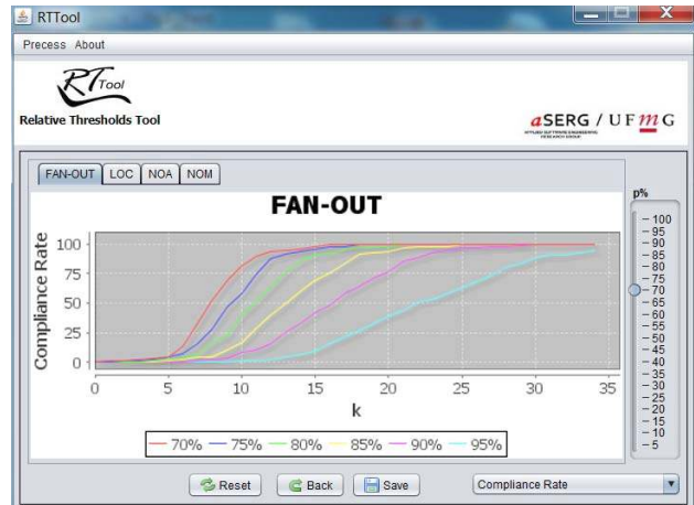
Fig. 5. ComplianceRate function (FAN-OUT metric)
