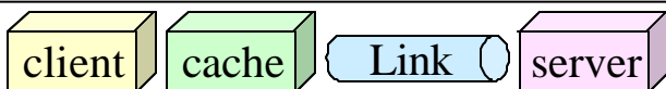
Figure 2. The client-side or proxy web cache improves response time by eliminate link transmission times and server times.
