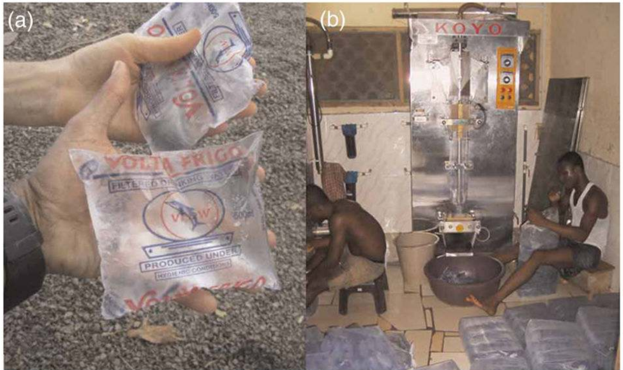
Figure 1. (a) Sachet water purchased from a street vendor, and (b) typical Koyo sachet filling machine at a small production facility in Accra.
