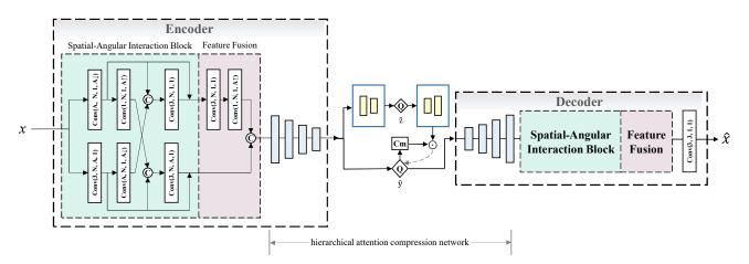
Fig. 2. Overview of the SADN architecture. The convolution layer is denoted as Conv (kernel size, channels, dilation, stride). A and N are 13 and 48 in our implementation respectively.
