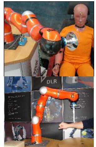
Fig. 3. Collision experiments with an LWR-III HIIII dummy (upper) and human (lower).
