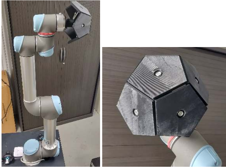
Fig. 3. (a) The UR5 robot with a prop attached to the end-effector and (b) The prop used to carry six sample textures. The lateral surface of the prop are denoted 1 to 5 and can be changed by a rotation of the last axis of the robot. The frontal surface of the prop is denoted 6. A displacement of the robot is required to present a lateral surface and then the frontal surface at the same cartesian location
