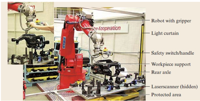
Fig. 3. Human-robot-cooperation for handling tasks. Inside a regular robot cell which is secured by light curtains, the robot handles gear boxes at regular speed in fully automated mode. Upon a human approaching the light curtain, the robot goes in the reduced-speed mode. The worker grasps the safety switch which activates the force-torque sensor. The worker guides the robot almost effortlessly by its handle [16]. (Fraunhofer IPA, Stuttgart)
