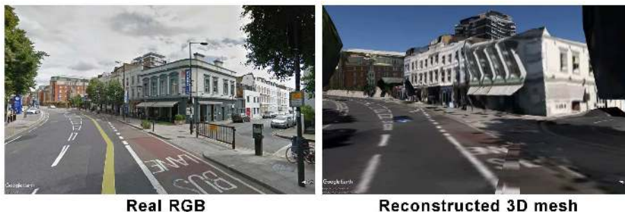
Fig. 4. A sample of RGB vs reconstructed 3D meshes (used for training) from the same location. Note the significant geometric, texture and illumination inconsistencies introduced by the reconstruction in contrast to a real-world capture. The darker regions in the right and left are tree meshes. While these meshes are very difficult to use for learning something at the ground level, from a birds’s eye viewpoint they look similar to the real RGB image.
