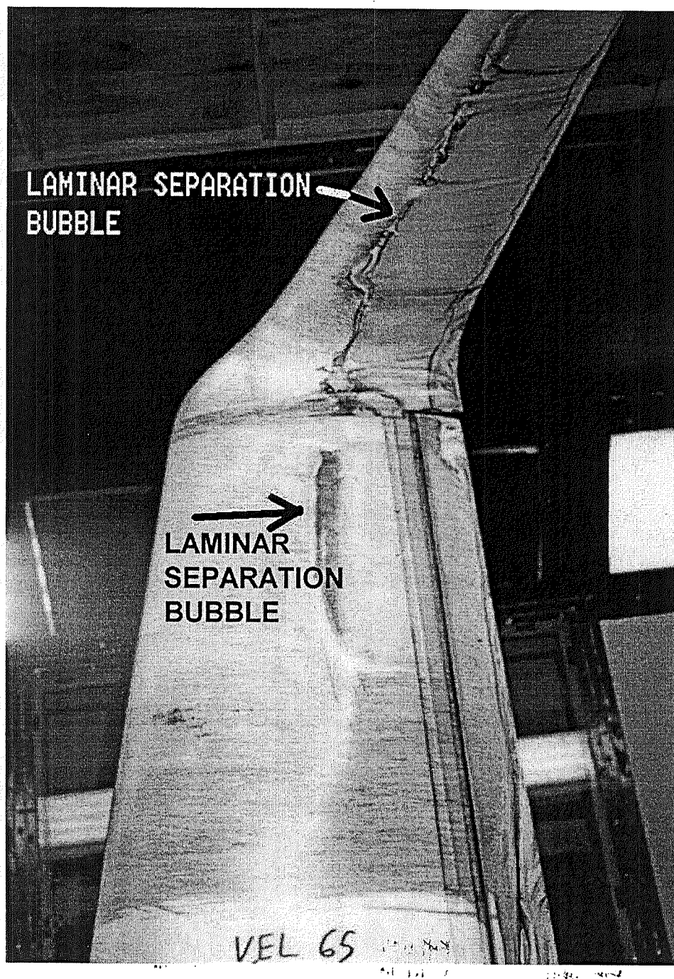
Figure 21. Flow Visualization of Winglet Suction Side. \alpha = 5.0^\circ , Q = 10.85 \text{ lb/ft}^2
