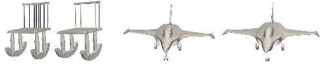
Figure 9: Failure in capturing thin structures. In each pair: ground truth model (left), and SAL reconstruction (right).
