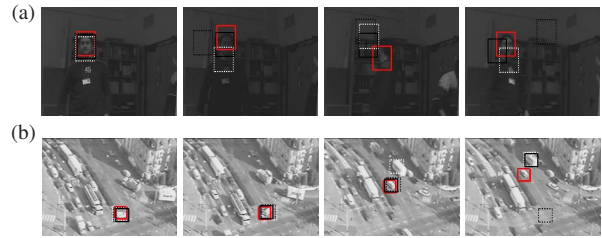
Figure 4. Results of tracking on a) “motinas_toni_change_ill” [22] - the person is turning around and the illumination changes drastically b) “karlsruhe” [1] - the car makes a U-turn. The target locations obtained by the four methods on four frames are shown : DST - thick red (pale gray when not in color) box, Collins - thick black box, ensemble - white dashed box, IVT black dashed box.
