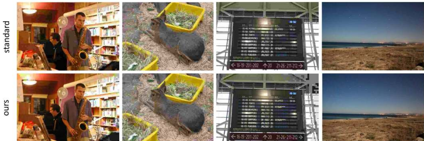
Fig. 3: Standard JPEG vs. our saliency-based variable coding results at the same bitrate. Some of the best parameter settings for the images in our collection with respect to DMOS. The salient parts of the image are considerably better quality than the less important and less noticeable background details. Refer to Table I for the parameters and study results for each image.
