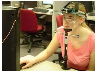
Fig. 8. Our experimental setup for the user study with the ISCAN ETL-500 eye-tracker.
