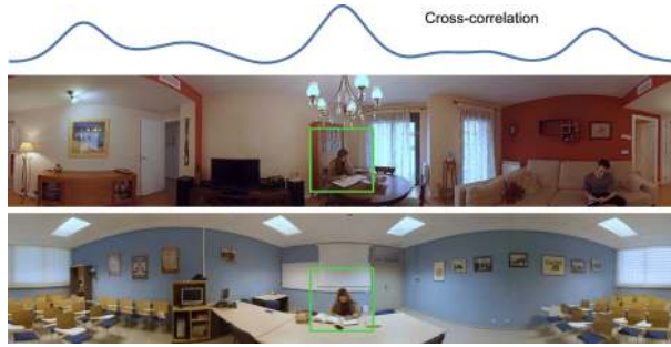
Fig. 10. Automatic alignment of cuts in VR video. To align two video segments, we can maximize the correlation between the saliency maps of the last frame in the first segment and the first frame of the second one. The cross-correlation accounting for all horizontal shifts is shown on top of this example, which has been automatically aligned with the proposed algorithm.
