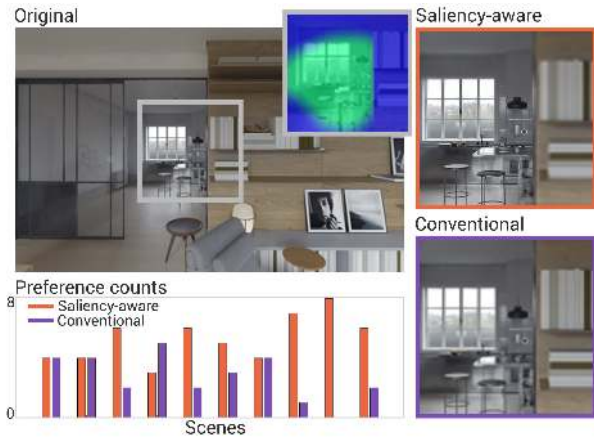
Fig. 13. Saliency-aware panorama compression. Top left : original, high-resolution region of the input panorama. Inset shows the compression map based on saliency information, where green indicates more salient regions. Right : Close-ups showing the differences between saliency-aware compression and conventional downsampling. Note that salient regions retain a better quality in our compression, while non-salient regions get more degraded. Bottom left : Preference counts for the ten scenes displayed during the user study.
