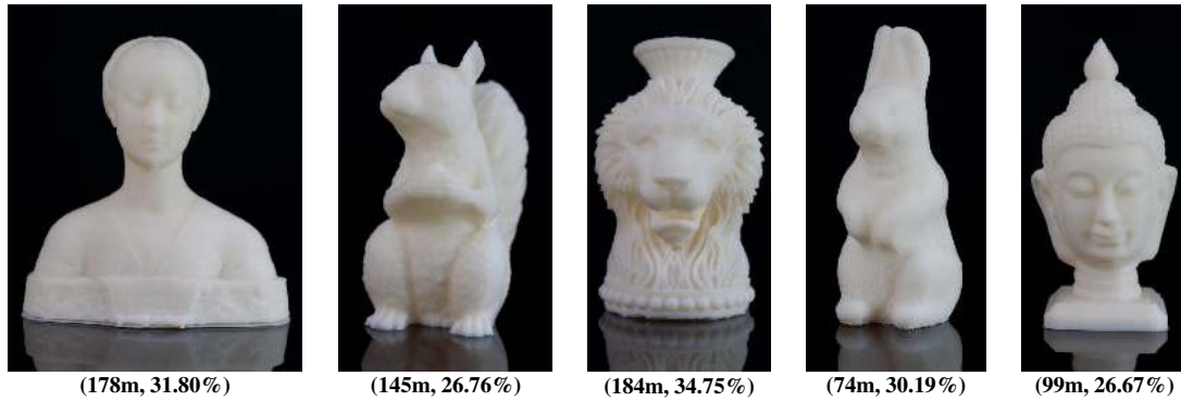
Figure 14: Photos of the printed objects using AdapSlice. Numbers in brackets below each photo denote its printing time (in minutes) and its ratio of time saving according to the ground truth. As shown in the user study, there is no apparent visual difference between these objects and their corresponding ground truth.
