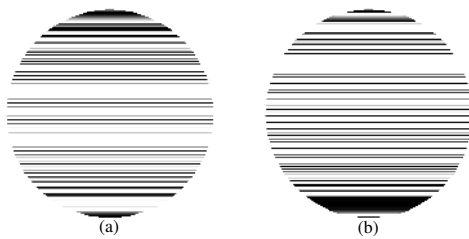
Figure 13: Slicing results on a sphere model using different methods. (a) The result produced by the method of [Dolenc and Makela 1994]; (b) The result produced by AdapSlice.
