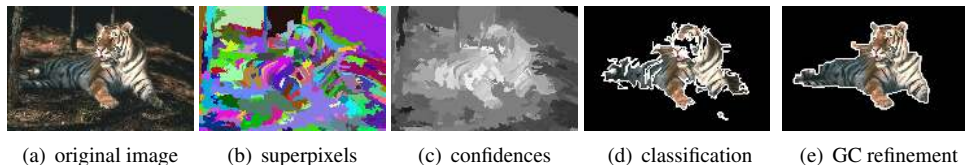
Figure 1: Summary of our approach. First the input image in (a) is segmented into superpixels, shown (b). Then the trained classifier is applied to each superpixel individually, classifier confidences are in (c). Based on confidences, superpixels are classified into salient/background, shown in (d). Finally the results in (d) are refined with graph-cut optimization, and the result after the refinement is in (e).
