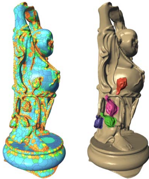
Fig. 1. Left: curvature analysis of the Buddha model and the local surface descriptors. Blue is low curvature and red is high. Right: the self-similarity of the four lotus flowers, which are detected by our partial matching technique.
