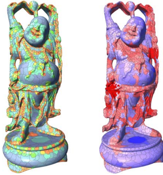
Fig. 9. The left image shows the local surface descriptors colored by the curvatures. In the image on the right the saliency grades are visualized on a scale from blue to red. The patches are colored according to the saliency grade of the salient feature that contains them.
