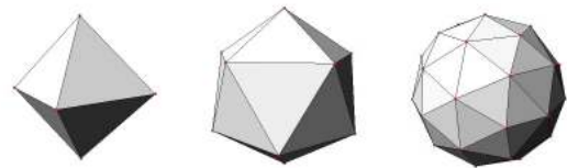
Figure 3. Cameras are placed at vertices of a polyhedron having either 6, 12, or 42 vertices, looking at the center of the polyhedron, for uniformly spaced (in terms of solid angle) view directions.
